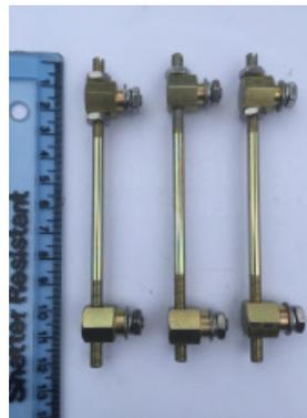
The linkages will not fit the PI systems fitted to later CR engine TR6 cars or 2.5PI saloon cars, or cars that have been retro fitted with CR or 2.5PI saloon car PI systems.
